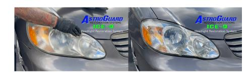
Clear coat will "set up" within 1-2 minutes. You can correct any streaks or bubbles during this time by lightly reapplying UV coating. The clear coat is usually dry to the touch within 10 minutes. The UV coating will be completely cured within 4 hours. Do not wash the car or expose to rain if possible for 24 hours.
