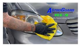
**Surface MUST** be **COMPLETELY** dry for proper clear coat adheision.
