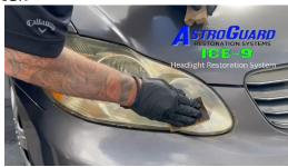
Step 3: Thoroughly wet the "white" clarifying sponge and scrub the entirety of the headlight for 30-40 seconds horizontally using firm pressure.
