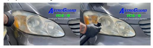
Step 2: While the oxidation removal spray is still on the headlight, lightly scrub the headlight moving horizontally with the "brown" sanding sponge for 30-40 seconds. Rinse with water.
